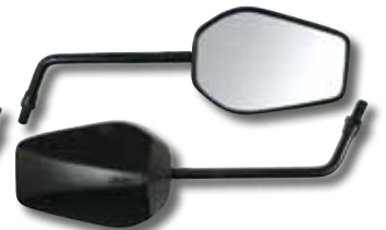
"Source" 10mm thread universal mirror. Fully E-marked, suitable for homologation projects. (PAIR) MRU016
