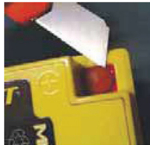
Removal of terminal plugs
