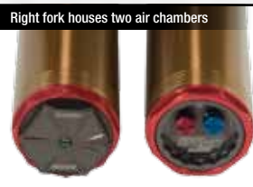
Right fork houses two air chambers
