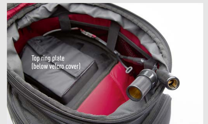
2 Cigarette lighter socket with SAE plug inside the electric tank bag
