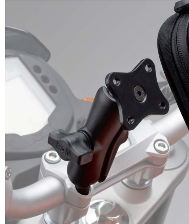
Ball, RAM arm 3" and universal mount installed to handlebar
