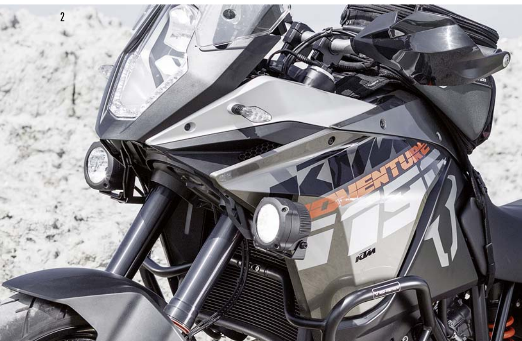
1-3 HAWK LED fog lights, 2+3 Mounted with light mount set (bike-specific), 4 HAWK light clamp (set includes 2 clamps with inlays for crash bars ø 22/26/27/28 mm)
