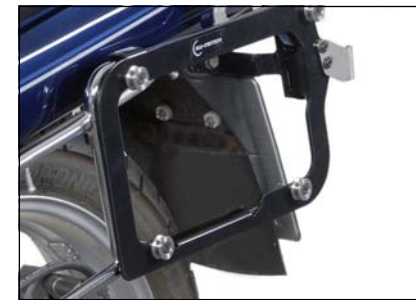
TraX® EVO/TRAX ADV side case adapter kit on Hepco & Becker side carrier
