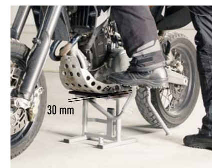
For optimal leverage a gap of ca. 30 mm is required prior to lifting
