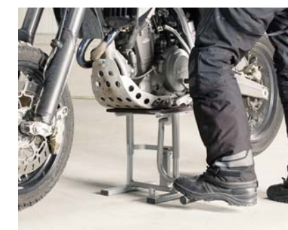
... then push down the lever until the motorcycle remains in the elevated position.
