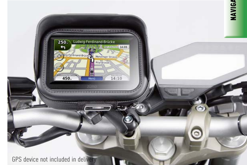
Handlebar mounting with RAM arm 3", universal mount and Navi Case Pro
